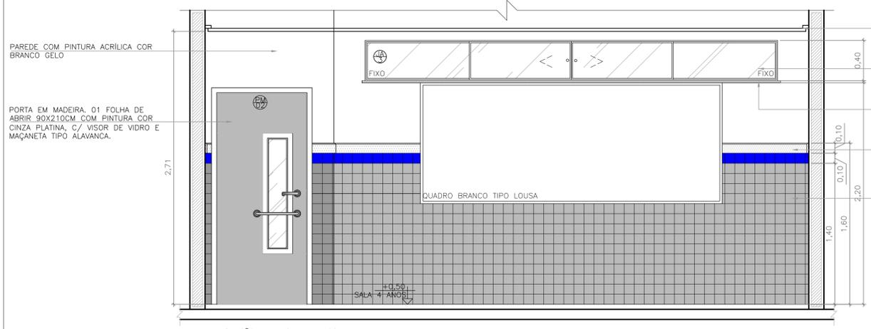
PORTA EM MADEIRA, 01 FOLHA DE ABRIR 90X210CM COM PINTURA COR CINZA PLATINA, C/ MAÇANETA TIPO ALAVANCA.
