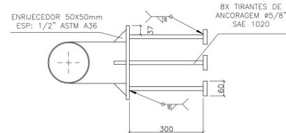
**DETALHES DO SUPORTE DE ANCORAGEM NO PILAR CENTRAL**
