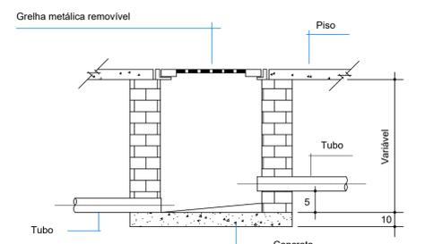
CORTEAA\_CAIXA DE PASSAGEM COM GRELHA S/ESCALA
