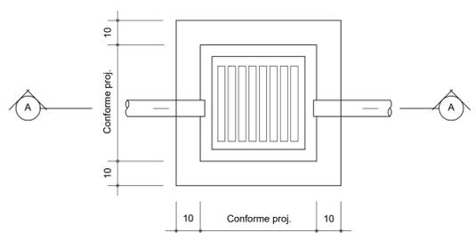
DETALHE - CAIXA DE PASSAGEM COM GRELHA S/ESCALA
