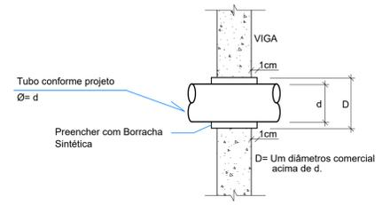
DETALHE - TUBO PASSANDO POR VIGA S/ESCALA
