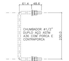
DETALHE DO CHUMBADOR DUPLO (TRELIÇA DO TELHADO) esc 1:5
